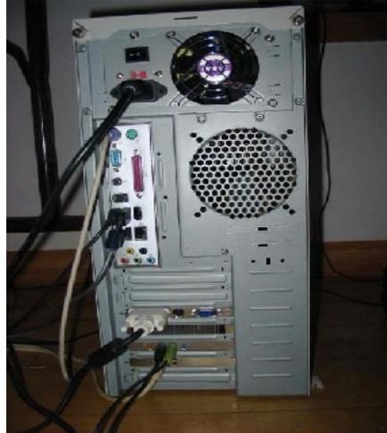
The first cable you will disconnect is the Power Cord, the one connected to the electrical outlet. After that is unplugged you can safely disconnect the other cables. I usually start with the top cables and work my way down, laying them on the floor in an orderly fashion. Also unplug the Electrical Cord to the Monitor.
