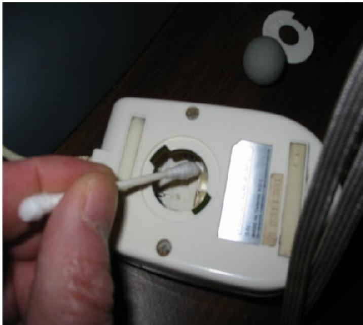
Next put some alcohol on a cloth and clean the rubber ball, then dry it. Once you are done cleaning, put the ball back in and then the ring, then twist the ring to lock it into position.
