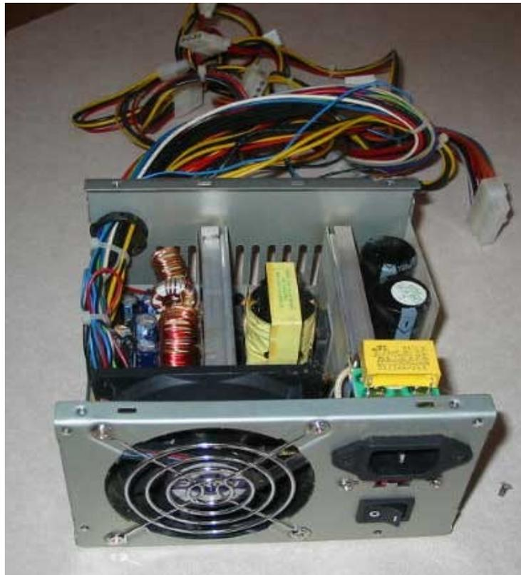
The only reason I am showing you this is to emphasize that this is the only thing that has Electricity stored when you unplug the Power Supply Cord from the computer and to take special care when cleaning it. As I said above only stick the small plastic tube that you attached to the can of compressed air into the Power Supply Box, do not over spray inside this box, just spray enough to clean out most of the dust.
