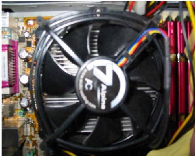
If you cannot get all the dust blown off the fan blades with the canned air, you can use a cotton swab to clean them. Once you have loosed up the dust use the can of air to blow off the excess.
